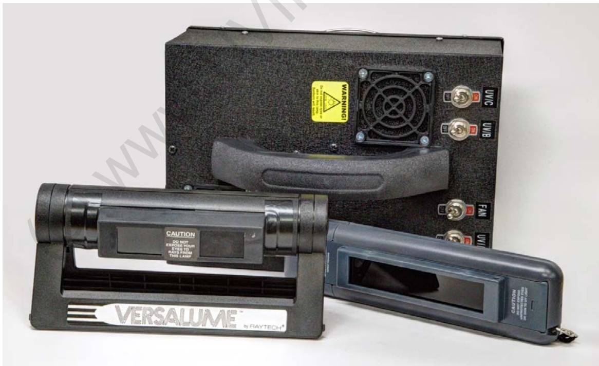
Figure 4 – Some popular UV lamps used by fluorescent mineral enthusiasts include the Versalume LW/SW (front), Spectroline MinMAX SW (middle), and pro-grade Way Too Cool 18 W LW/MW/SW filtered UV sources.
